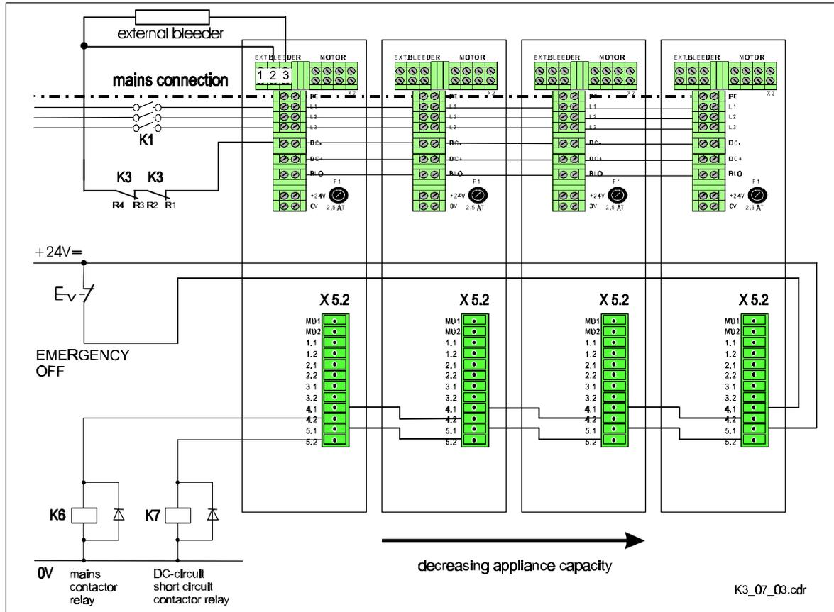
Wiring (external bleeder): as above, but with connection to 16A or 25A compact appliance
