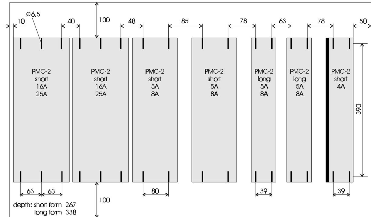
Installation scheme for the motor filter with minimum distances
