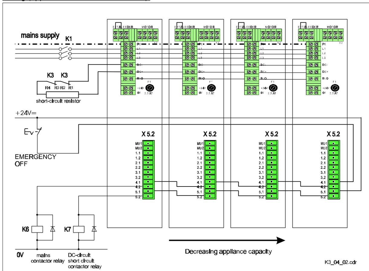
Wiring (external bleeder): Bleeder is at the same time DC-circuit short circuit resistance
